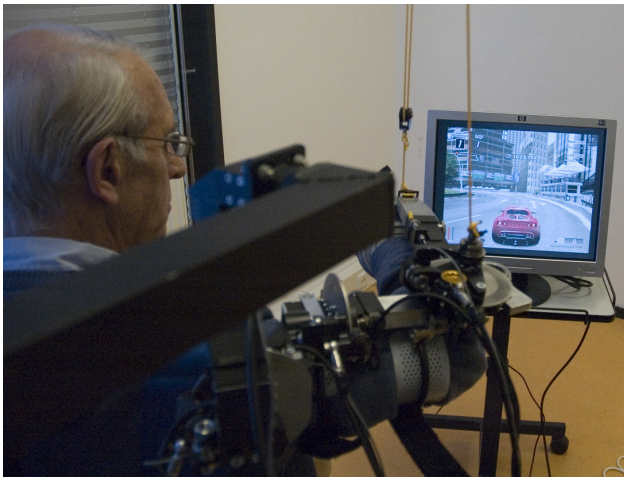
Fig. 6. Integrated gaming environment connected to Dampace torques and movements. Either isometric thoracohumeral-elevation torques or isotone rotations are mapped to the gas paddle in the racing game, and either humeroulnar isometric torques or isotone rotations to the steering wheel. Good coordination of simultaneous shoulder and elbow torques is thus required for good driving control in the game and should motivate the subjects to keep exercising.
