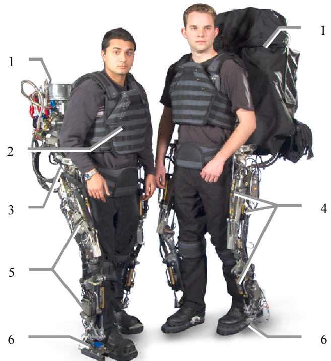
Fig. 1 Berkeley Lower Extremity Exoskeleton (BLEEX) first generation prototype and pilot. 1: Hydraulic power supply and payload occupies the upper portion of the backpack; 2: Rigid BLEEX spine connected to the flexible pilot vest; 3: Central control computer occupies the lower portion of the backpack; 4: Some of the hydraulic actuators (ankle, knee and hip); 5: Two of the control network's Remote I/O Modules (RIOM); 6: Rigid connection of the BLEEX feet to the pilot's boots. More photographs can be found at http://bleex.me.berkeley.edu
