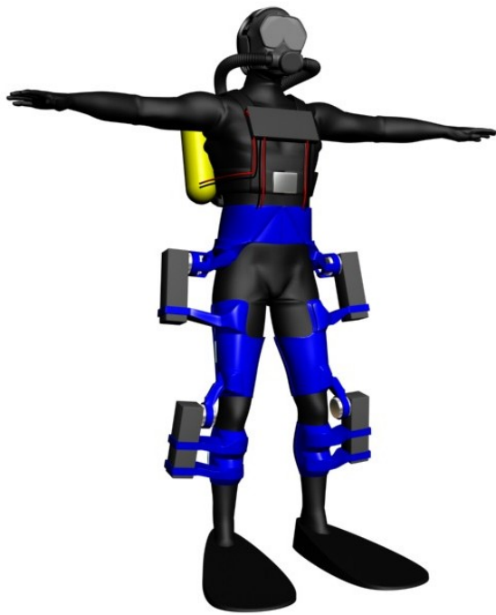
Figure 1 Concept drawing of lower extremity exoskeleton, front view. Rotary motors are shown actuating the knee joint and hip joint.
