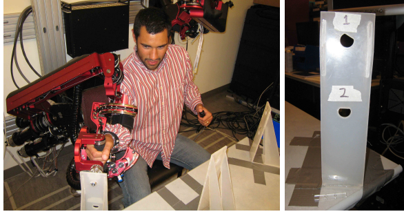
Fig. 4. A subject inserts the tip of the exoskeleton into a target. There was a total of 6 targets. Each subject performed 4 repetitions of every controller moving to every target
