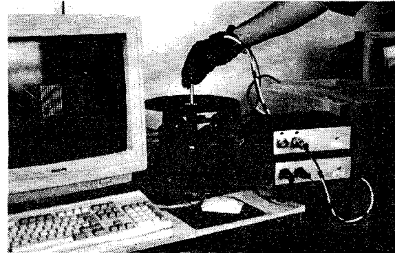
Fig. 5. Operation of Impulse Engine while wearing the Tactile Glove
