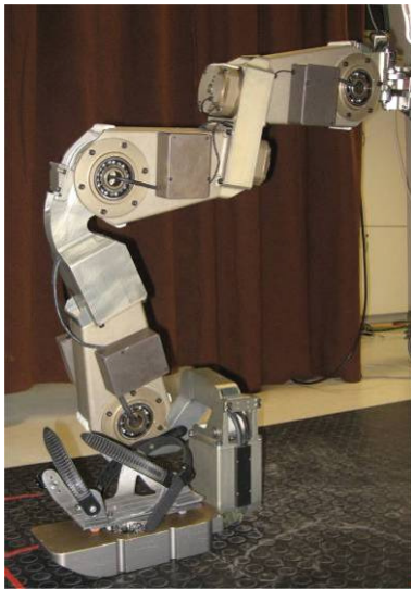
Fig. 7. Three transversal joints integrated for the implementation of the PERCRO BE right leg.
