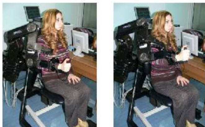
(a) The starting position of the reaching task. (b) A subject in the middle of the path of the reaching task
