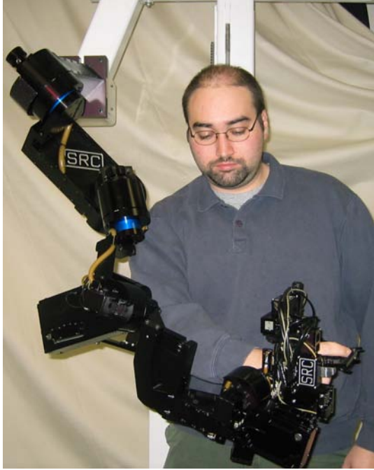
Fig. 1. Sarcos Master Arm with user.
