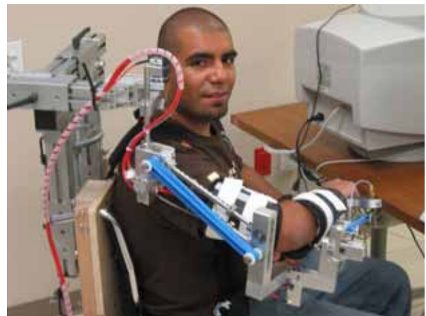
Figure 1: T-WREX. The orthosis provides gradable support for the arm against gravity using elastic bands, and measures arm movement and hand grasp as the user interacts with computer simulations of functional activities.
