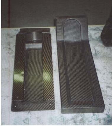
Figure 7. Example of a link and its die made of carbon fiber
