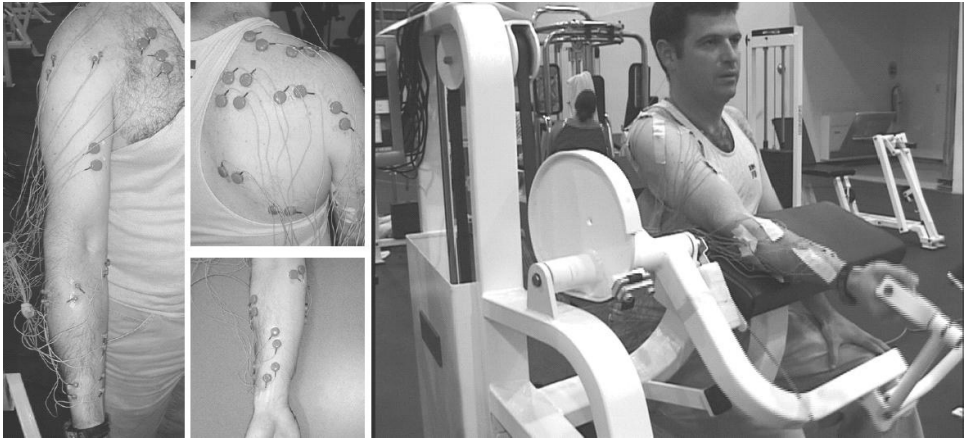
Fig. 5. Experimental setup for measuring neural activity (sEMG) along with the kinematics and dynamics of selected arm activities (e.g. flexion and extension of the elbow) under various loading conditions.
