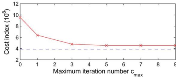
Fig. 4. Total performance cost along the closed-loop system trajectories of centralized LMPC (dashed line) and iterative DMPC (solid line).
