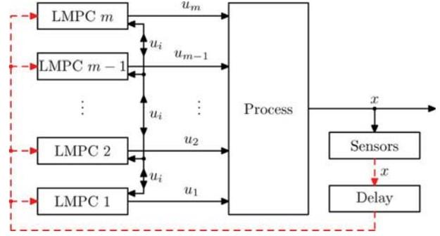
Fig. 1. Iterative DMPC with asynchronous, delayed measurements.
