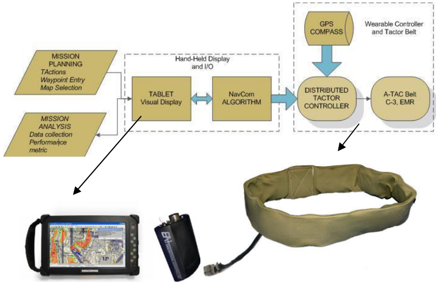
Fig. 4. Block diagram for the proposed ATAC-NavCom system
