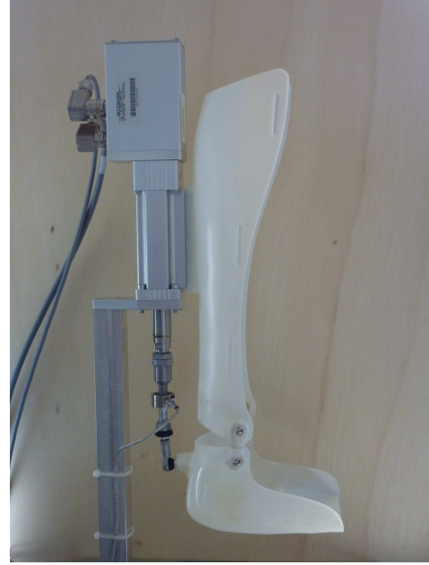
Fig. 6: Foot elevator orthosis aims at elevating the foot after the toe off.
