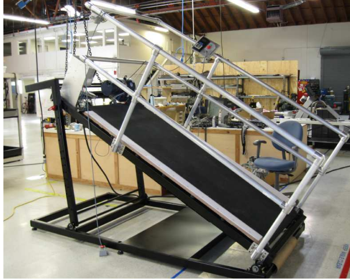
Figure 6. Assembled treadmill with safety covers removed.
