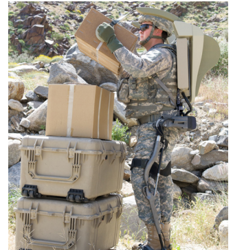
Allows One Soldier to Lift Loads, Maintains Normal Lifting Range of Motion and Keeps the Center of Gravity Close to the Soldier
